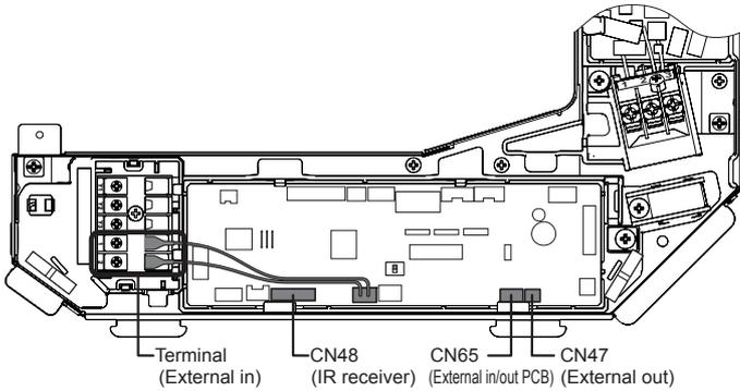
This air conditioner can be connected with the following optional kits. For details on how to install optional parts, refer to the installation manual included in each item.
