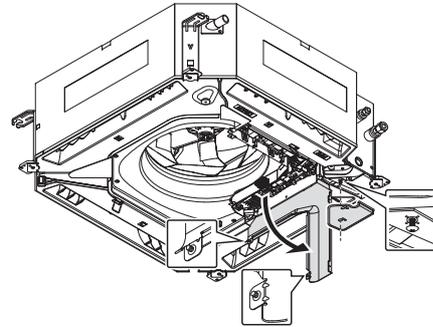
(2) Thread each cable through the holes or indents of the cabinet and connect the wires.
