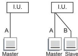
A, B : Remote controller cable. (Refer to 2.4. Electrical requirement.)
