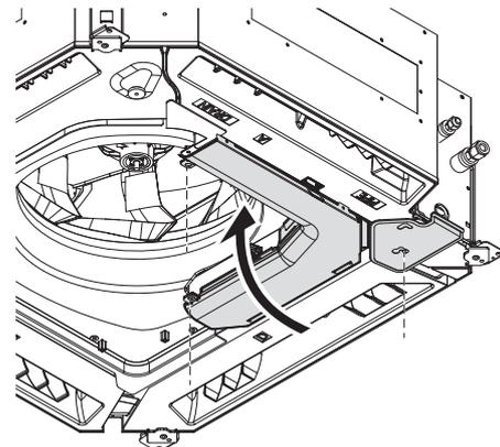
※ Cure the wiring connecting port and remote controller connecting port with paste or heat insulation so that insects or dust will not enter the unit
