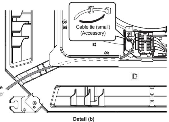
(4) Replace the Control box cover and Wiring cover. Securely tighten the screws.
