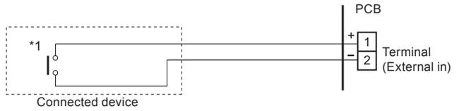
\*1: The switch can be used on the following condition: DC 12 V to 24 V, 1 mA to 15 mA.
