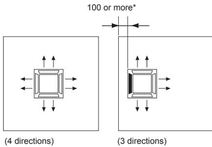
\* Please ensure sufficient service access during installation.
